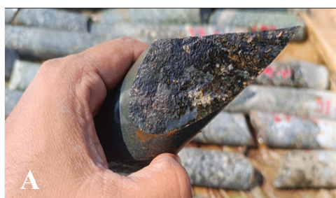
A. Dessiminations of Chalcopyrite, pyrite in Hand specimen of Borehole core sample (MSC-02) B. Photomicrograph of Polished section with Chalcopyrite (MSC-01)
