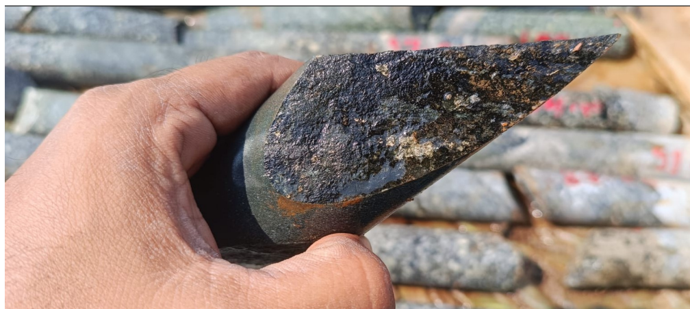
Photo 7.11: MSC-02 core showing dessiminations of pyrite, chalcopryite in granodiorite gneiss fracture plane
