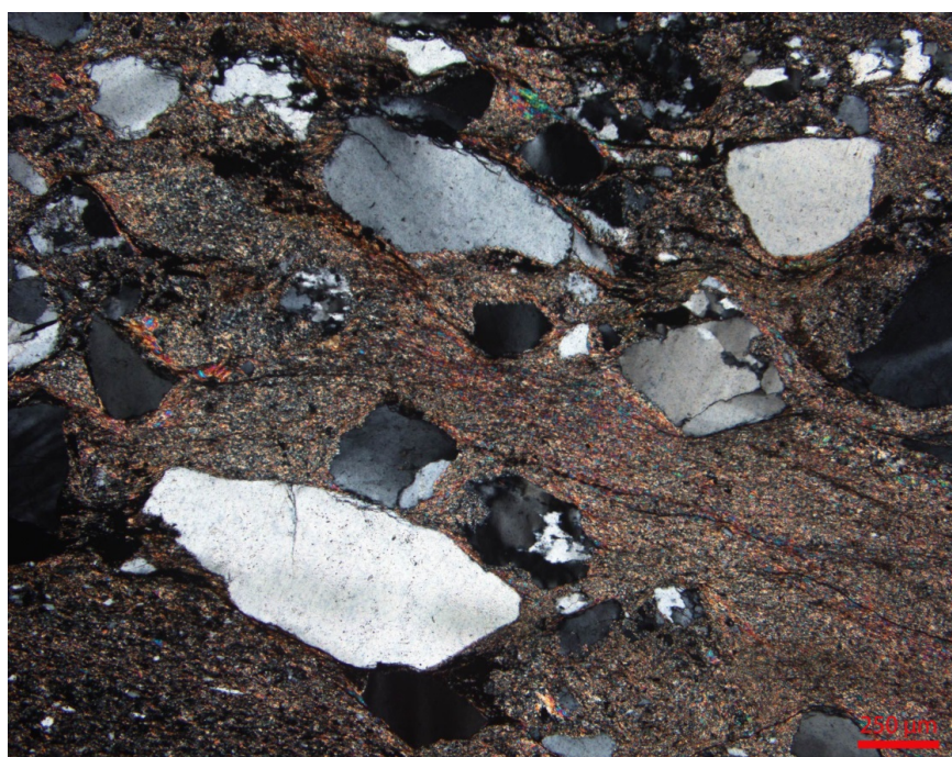
Pmg – 1: Photomicrograph showing association and parallel alignment of lensoidal and subrounded quartz and very fine sericite aggregates in quartz-sericite schist/ (mylonite?) as seen under crossed nicols.
